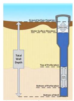
Figure 4-1: Well Completion Diagram
