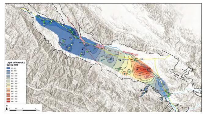
Figure ES-4: Depth-to-Groundwater in Spring 2018
