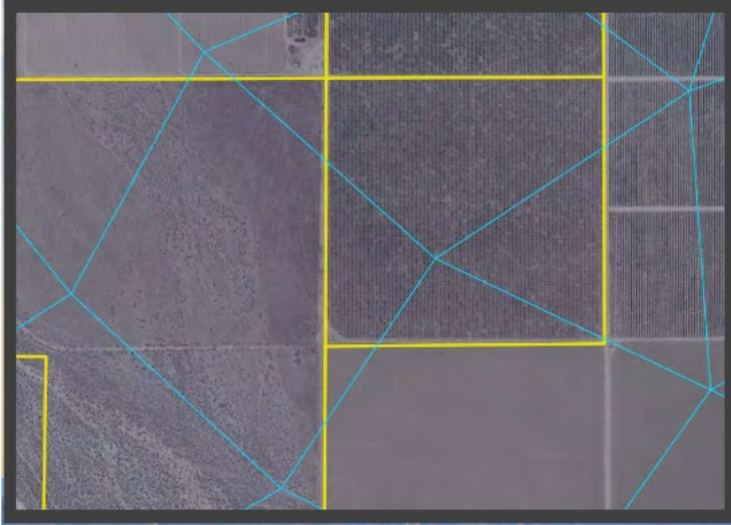
Figure 3. Example of CBWRM Model Elements (in blue) Overlain on Parcels (in yellow)
