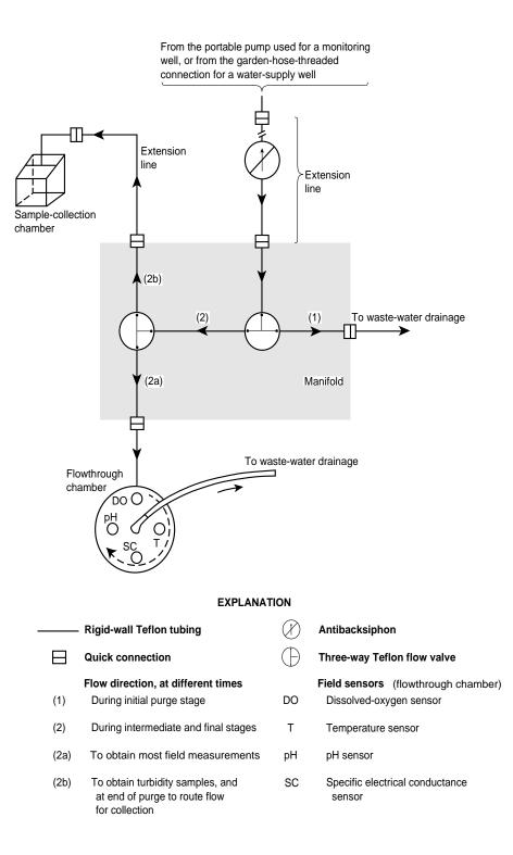
Figure 2. Schematic of equipment setup for well purge and sample collection.
