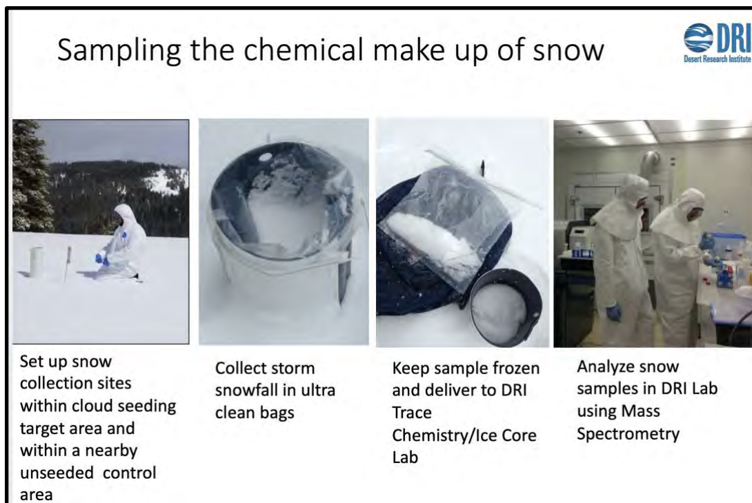
Figure 19: DRI snow chemistry collection and analysis methods
