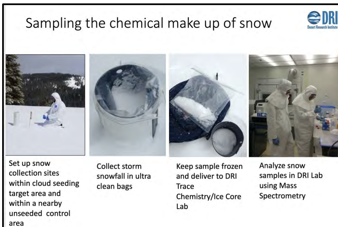
Figure 19: DRI snow chemistry collection and analysis methods
